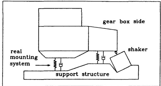
Fig 7: scheme of excitation system used for engine modal testing
