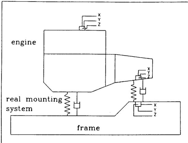
Fig 1: engine instrumentation layout during operational test
