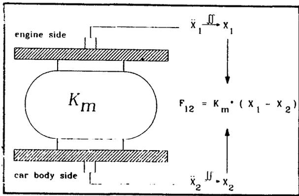
Fig 5: calculation of the force transmitted through the elastic support
