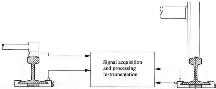
Fig. 6 Measurement scheme for FRF and train accelerations
