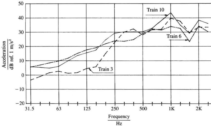
Fig. 10 Acceleration spectrum point 1 caused by trains 3, 6, 10
