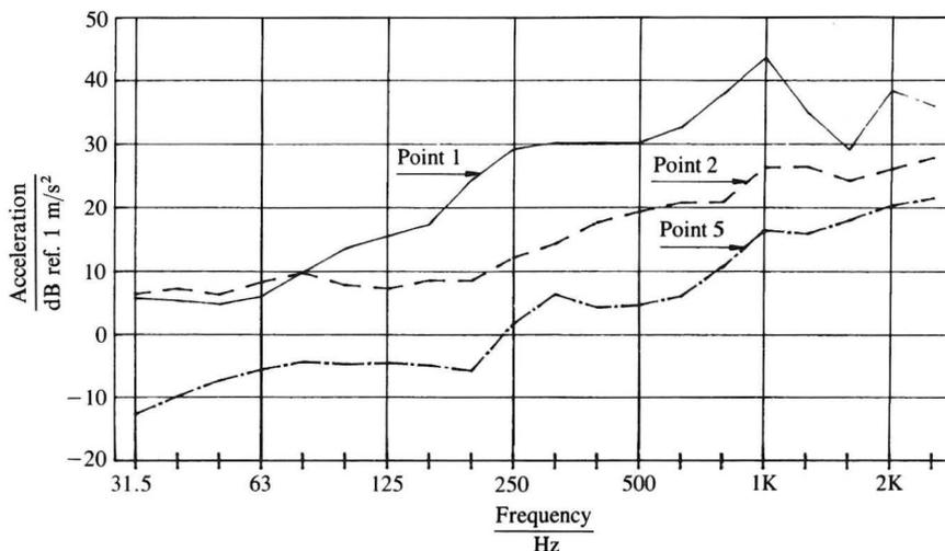
Fig. 11 Acceleration spectra points 1, 2 and 5 caused by train 10
