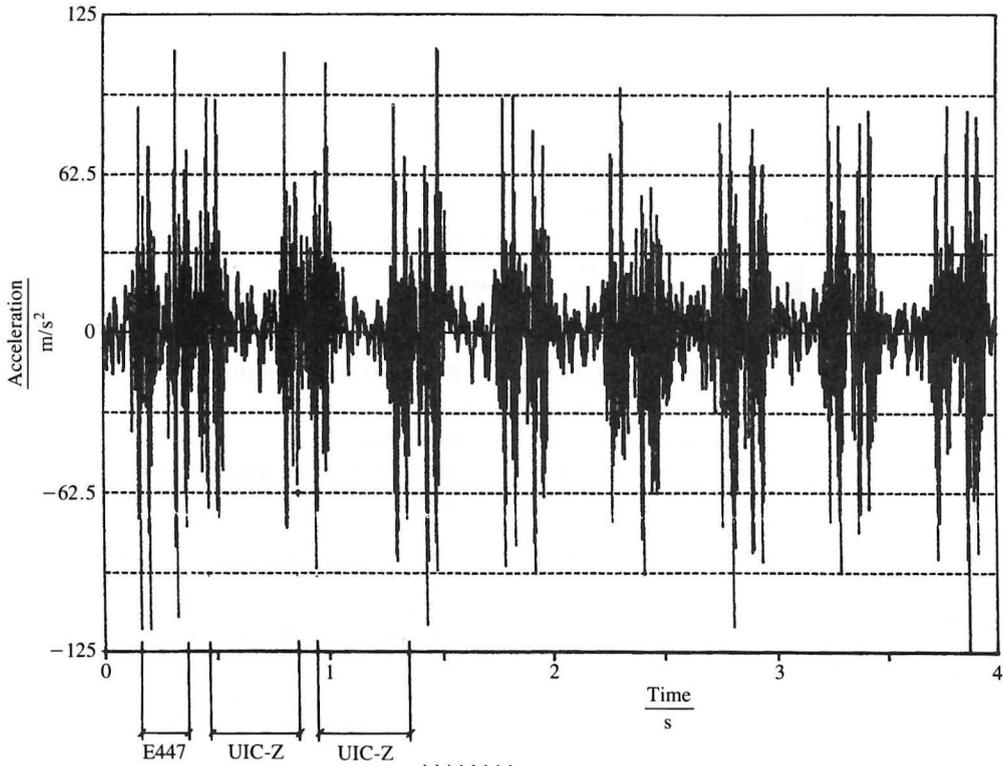
Fig. 8 Acceleration point 1 caused by train 10 ( $T = 4$  s)
