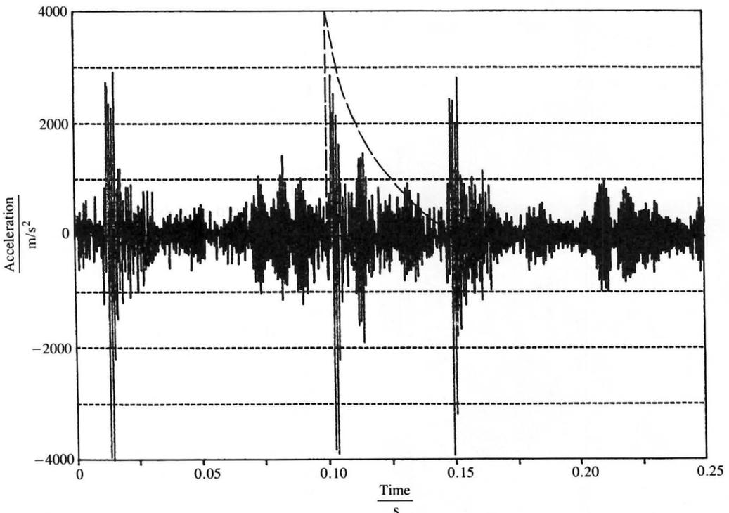
Fig. 9 Acceleration point 1 caused by train 10 ( $T = 0.25$  s)
