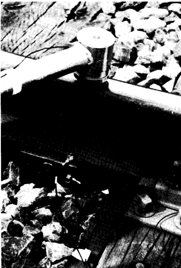
Fig. 7 Application of shock excitation on the track
