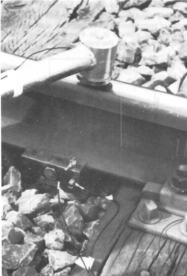
Fig. 7 Application of shock excitation on the track
