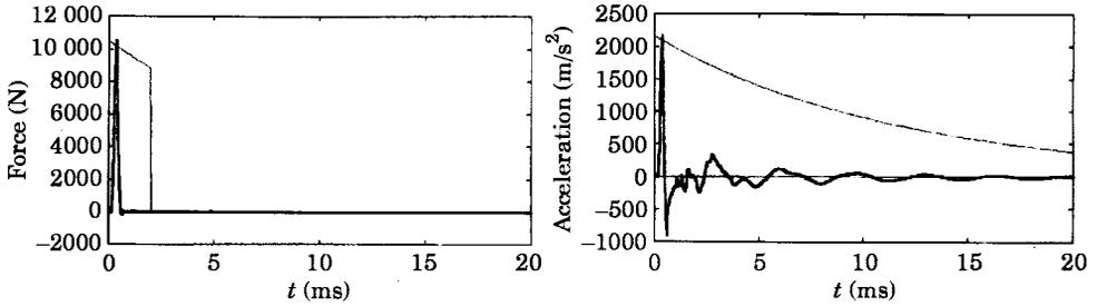
Figure 2. Time history of a hammer blow in the excitation point 1 and of the accelerometer signal in the same section (—) and time windows used for weighting (---). Time is limited to 512 samples, while the complete acquisition lasts 2048 samples.
