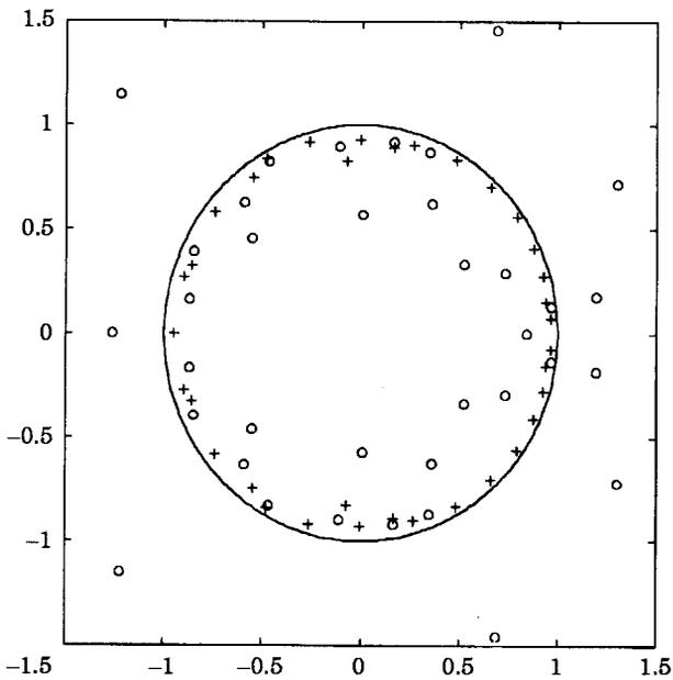
Figure 6. Poles (+) and zeros (O) of FRF  $H_{1,12}$  on the  $z$ -plane.
