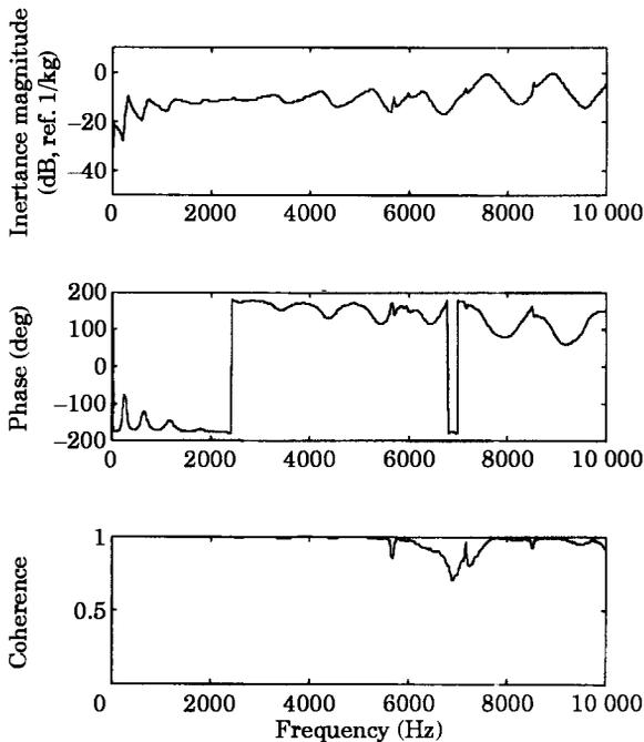
Figure 3. Magnitude, phase and coherence (six averages) of point FRF  $H_{1,1}$ . The frequency content of both force and acceleration signal is particular high in the whole range, as highlighted by the very good value of the coherence function.
