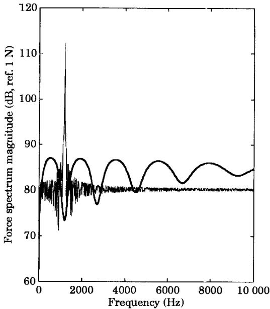
Figure 7. Magnitude of narrow- and broadband input signals applied to the system. Phases (not shown) are random. The energy of the two signals is similar.
