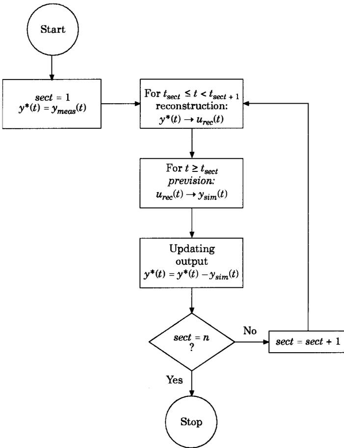
Figure 9. Block diagram of reconstruction algorithm (HF-MIRA).
