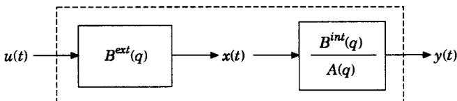
Figure 10. Block diagram of the system with  $B(q)$  decomposition and auxiliary time series  $x(t)$ .
