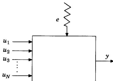
Figure 4. Block diagram of a MISO system in presence of extraneous noise or unmeasured input.
