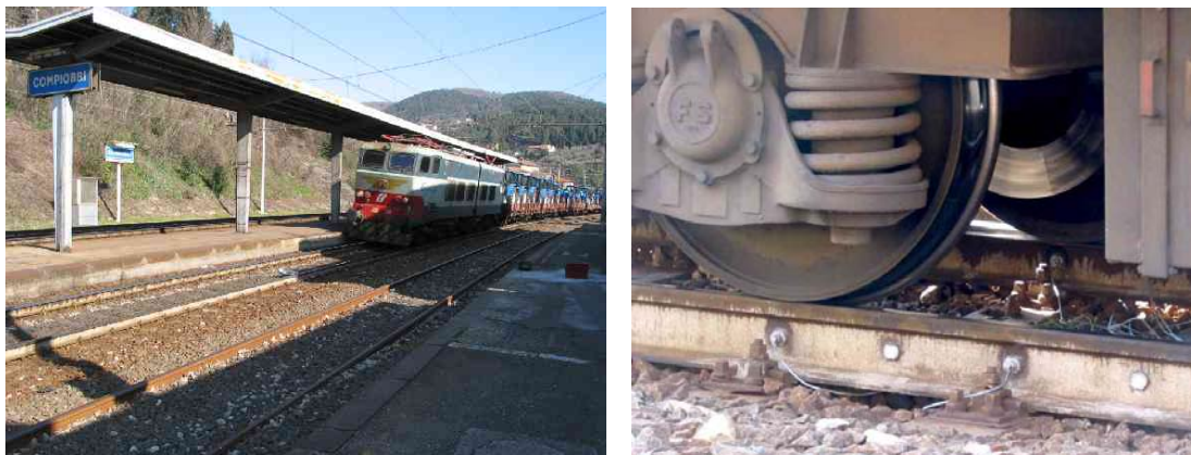
Figure 6. A freight train running at 90 km/h is approaching the measurement section (left); a regional train stopped just over the sensor (note the high level of railhead wear on the opposite high rail) (right).
