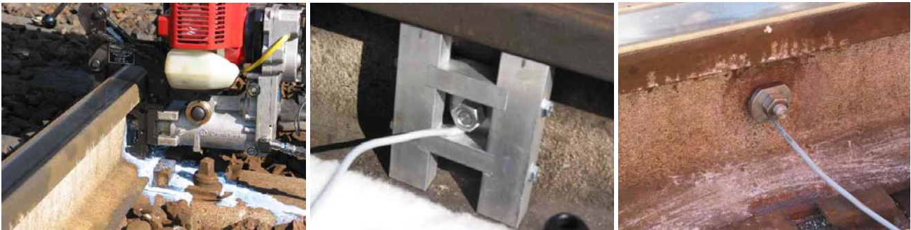
Figure 5. Mounting sequence of a sensor: drilling the rail (left), mounting the sensor with the appropriate mask, the final aspect of the sensor before sealing with silicon rubber
