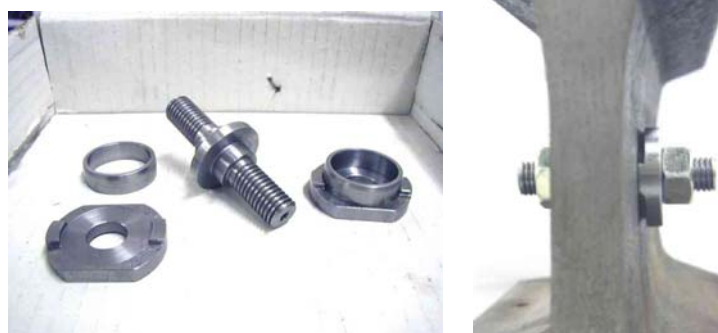
Figure 4. Mechanical parts (nuts not shown) of new sensor before application of strain gauges (left). Final mounting on the rail web, still without wiring (right)
