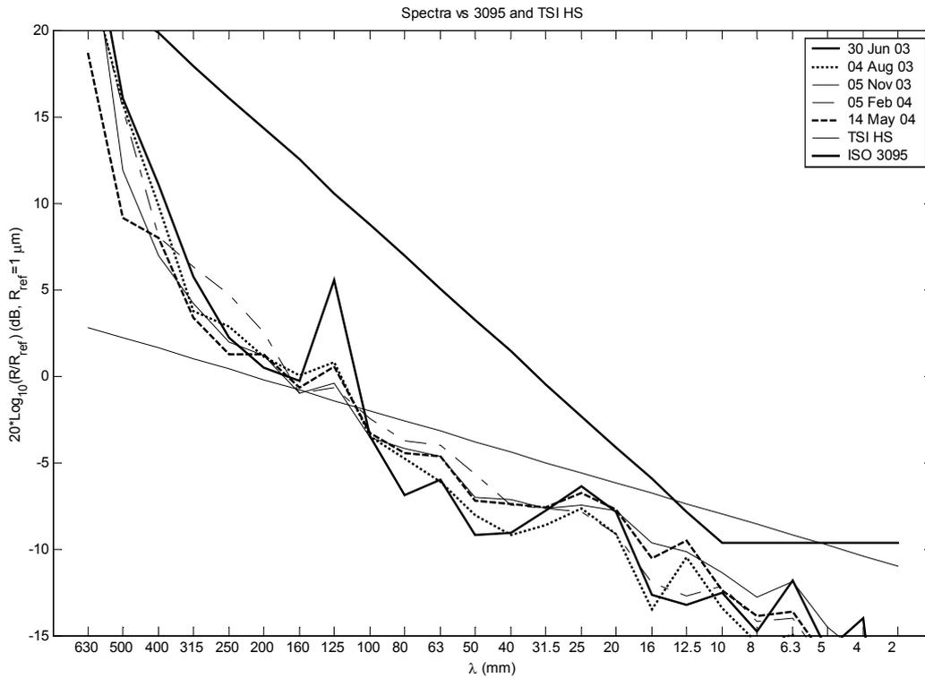
Figure 8. Spectral analysis of *leftcentre* (above, meas # 1,2,5,8,12, sections 410 to 567) and *rightcentre* (below, meas # 1,2,5,8,11, section 721 to 913) traces compared to ISO 3095 and TSI HS limits..
