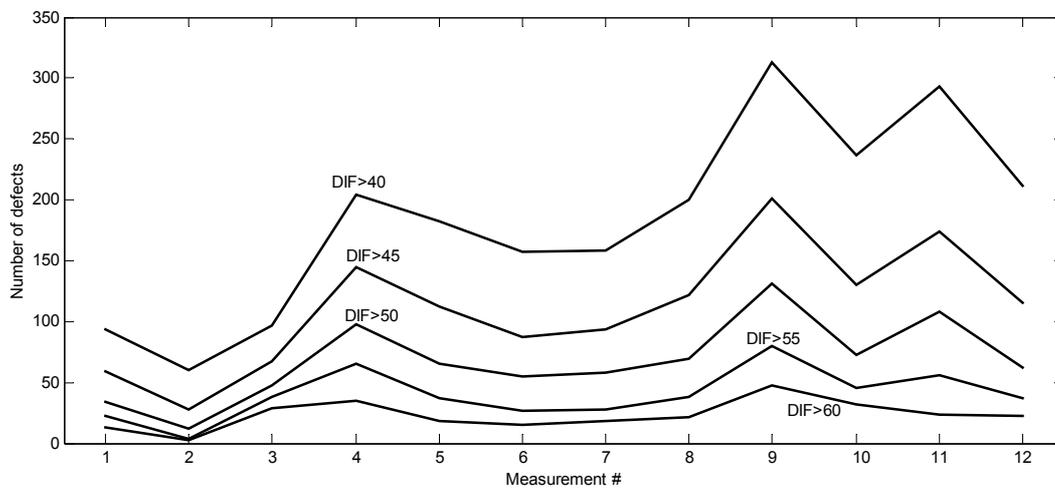
Figure 6. Number of defects found using the *DIF* criterion with indicated values for all *leftcentre* measurements.
