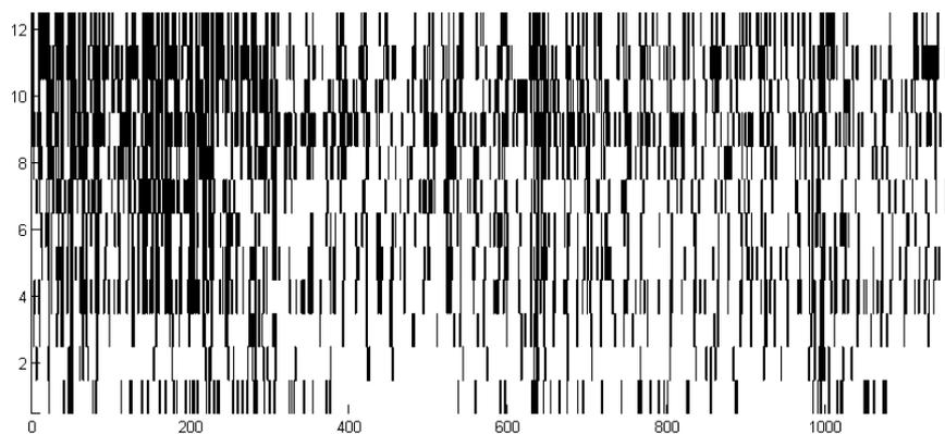
Figure 7. Defective sections found with *DIF*>40 criterion for all *leftcentre* measurements (x-axis: section, y-axis: measurement number).
