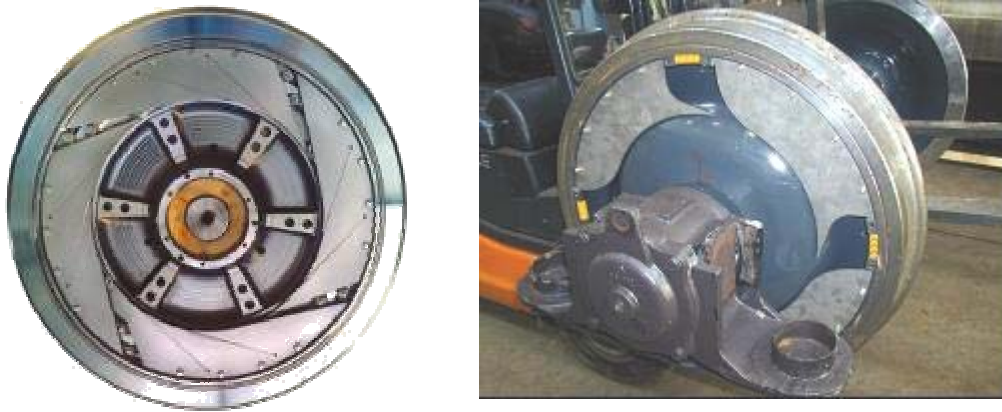
Figure 2 – Application of the Galene ® treatment to a tram vehicle (Siemens Combino ® , left) and to a low residual stresses wheel for freight wagons with tread braking (right)
