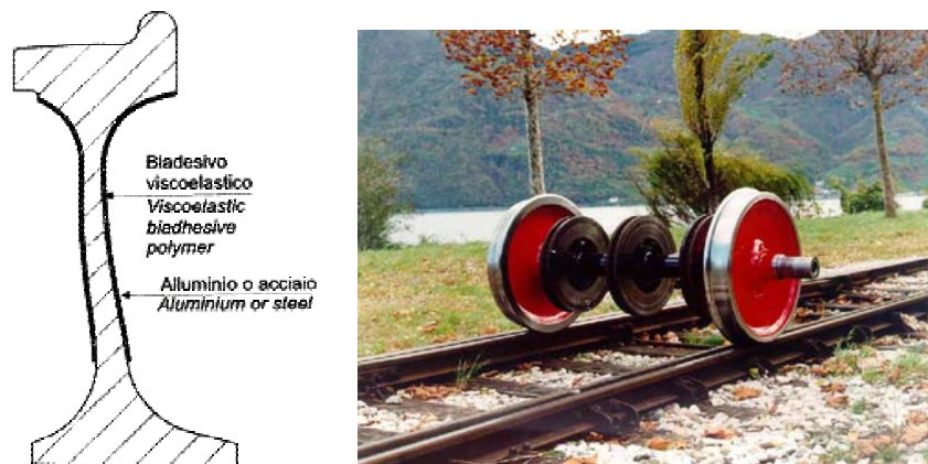
Figure 1 – Layout of the Syope ® damping treatment (left) and the first wheelset equipped with Syope ® treatment in the Lucchini Lovere plant in 1997 (right).
