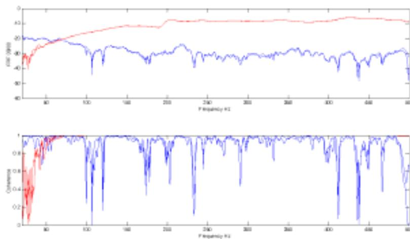
Figure 5. FRF and relative coherence function estimated with impact excitation on the rail and response recorded on the tunnel wall, for “slab track” (red) and “floating slab track” (blue).
