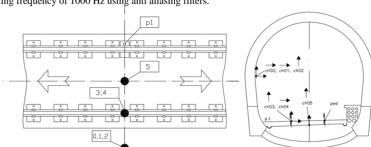
Figure 3 Location of accelerometers on track and tunnel (left: top view, right: cross section)
