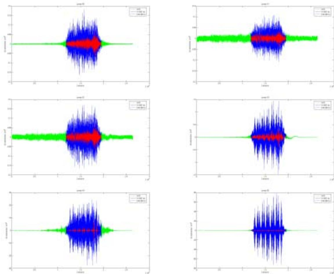
Figure 4. Time histories of acceleration on the instrumented points (slab track): wall horizontal (top left), wall vertical (top right), wall horizontal (backup sensor, mid left), slab vertical (mid right), rail horizontal (bottom left), rail vertical (bottom right). Green plot is all the signal in all the frequency range, blue plot is the portion of the signal used to calculate RMS, red is the same portion in the 0.8÷80 Hz frequency range.
