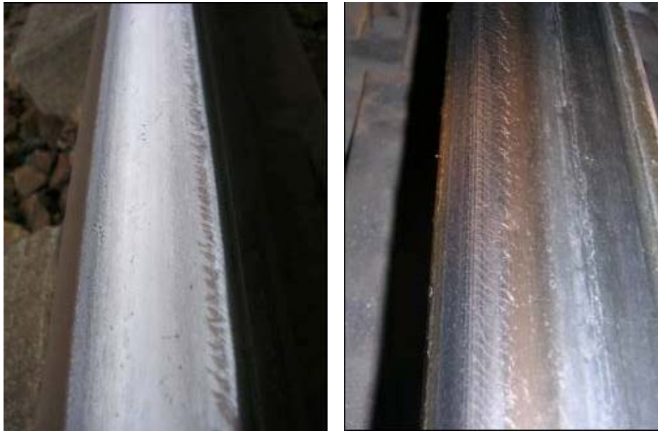
Figure 4. Head checks on R350HT ultra-hard rails on curve 49 (R= 356 m, h= 130 mm, left) and on curve 57 (R=491, h=120mm, right)
