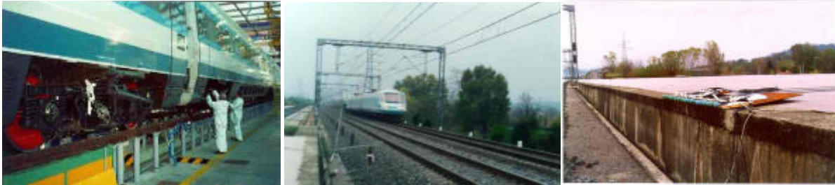
Figure 2. Left to right: experimental Syope ® wheels on the ETR470-0 trainset, trackside microphones during a 250 km/h pass-by, preparation of linear array of microphones.
