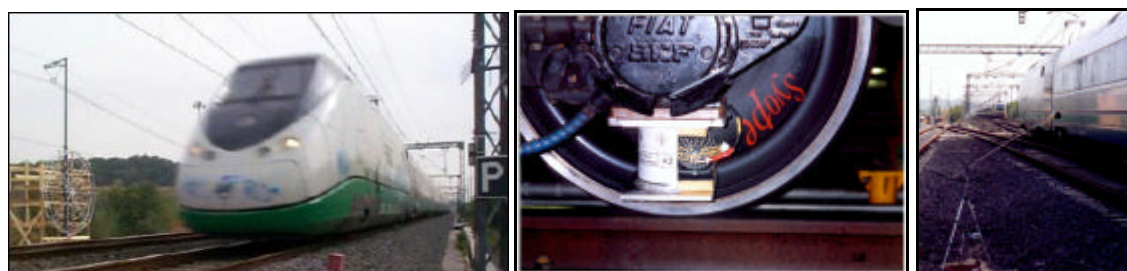
Figure 6: Some images from the test campaign in Renacci, 2000, on the ETR500 PLT trainset 51. Left: train passing by in front of the spiral array of microphones by DB; mid: axlebox noise measuring device developed by University of Florence in front of a Syope ® wheel; right: classical standing microphone at d=7.5m , h=1.2m from the track centerline.
