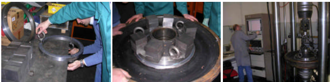
Figure 12. Tear test preparation. Left: the glue is applied to the internal ring. Mid: curing time was min. 24 hours. Right: Universal traction machine with Syope wheel mounted ready for tear test.
