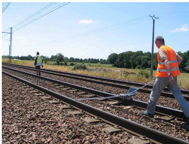
Figure 4. Snapshot taken while pushing the trolley at around at 2 m/s, the maximum safe speed that can be sustained on a ballasted track with bi-bloc sleepers.
