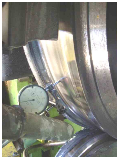
Figure 6: OOR measurement with 0.01 mm dial gauge.
