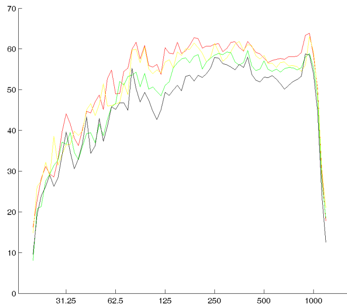
Figure 4: RMS average spectra [dB ref 20 \mu Pa] divided for noise category: black= normal noise , green= slightly noisier , yellow= noisier , red= much noisier .
