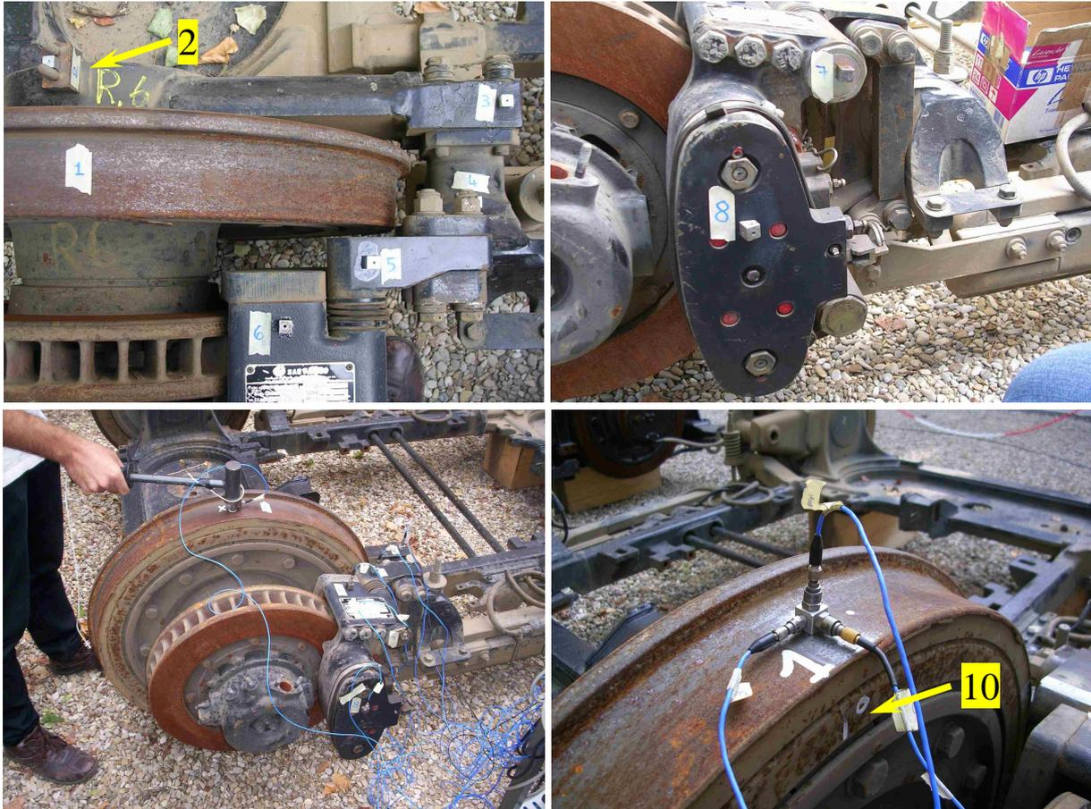
Figure 7. Measurement set up on the *original* calliper support assembly. Point numbering and definition: point 1: wheel tread, point 2: bogie frame, point 3: end of support arm, point 5: calliper fixture, point 6: calliper upper surface, point 7: calliper support side surface, point 8: calliper side surface, point 10: wheel web.
