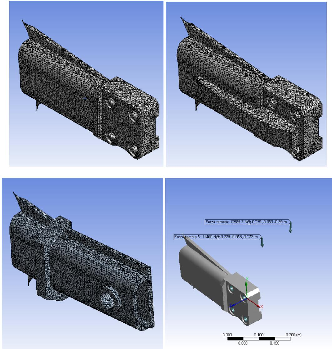
Figure 2. Finite elements models of the *original* (top left), *reinforced* (top right) and *modified* (bottom left) brake calliper support arm; loads applied on the original support arm (bottom right).
