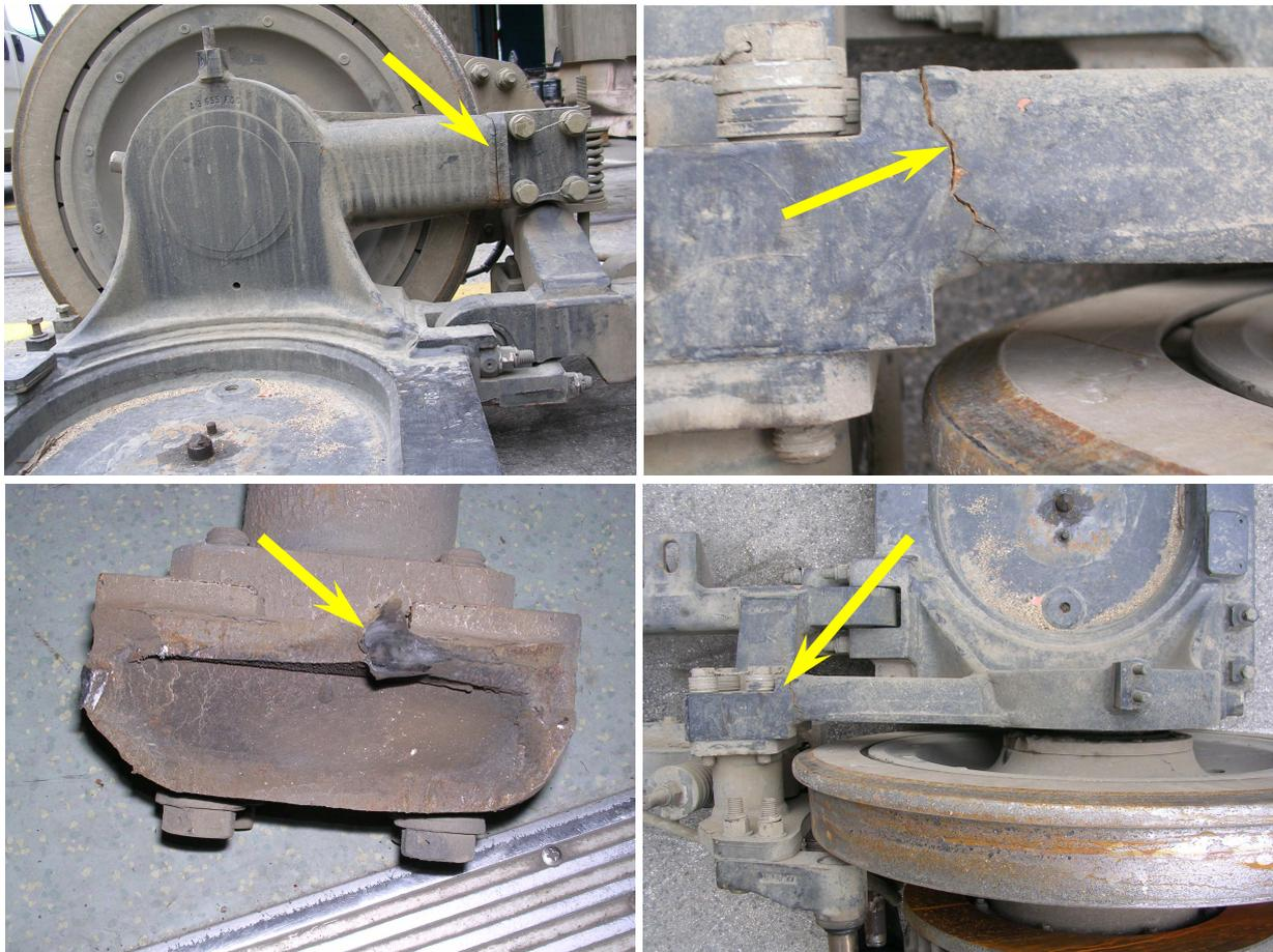
Figure 1. Some example of cracks and fractured surfaces on the brake arm.
