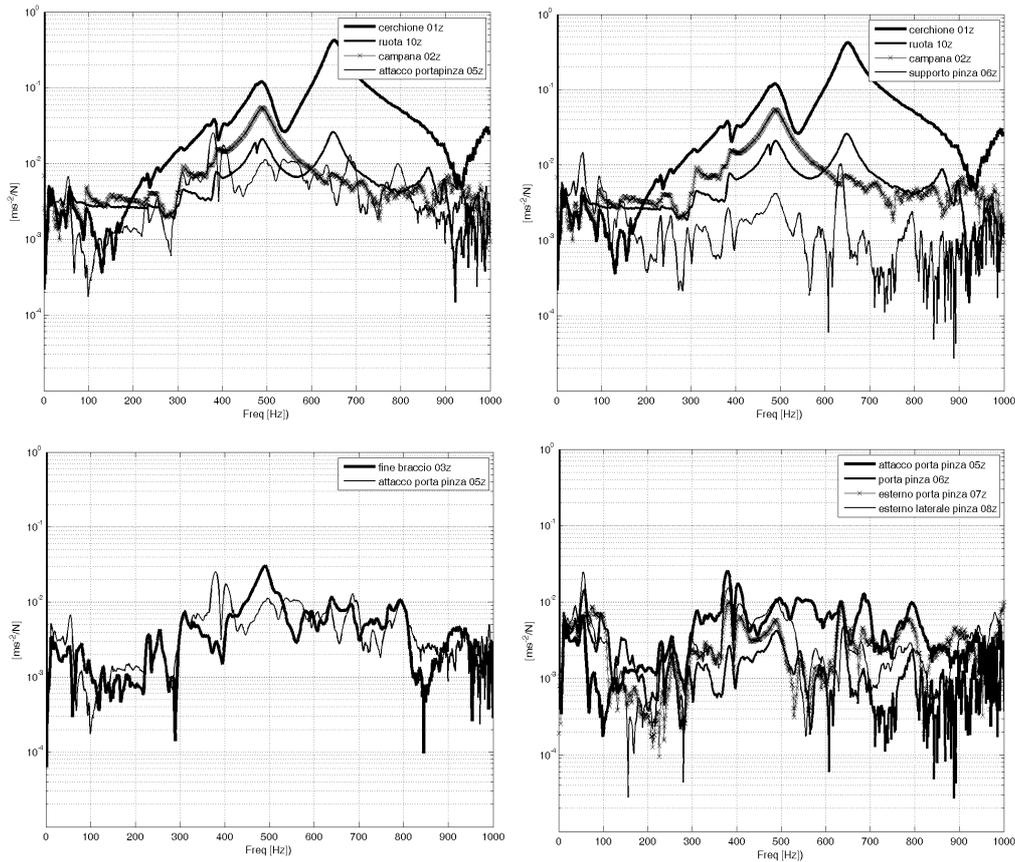
Figure 8. FRF for input on wheel tread (point 01z) and output on points 01z, 10z, 02z and 05z (top left), on points 01z, 10z, 02z and 05z (top right), on points 03z and 05z (bottom left) and on point 05z, 06z, 07z and 08z (bottom right).
