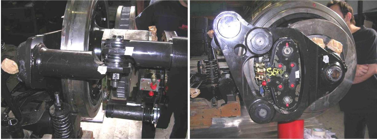
Figure 6. Redesigned calliper support assembly during laboratory tests.
