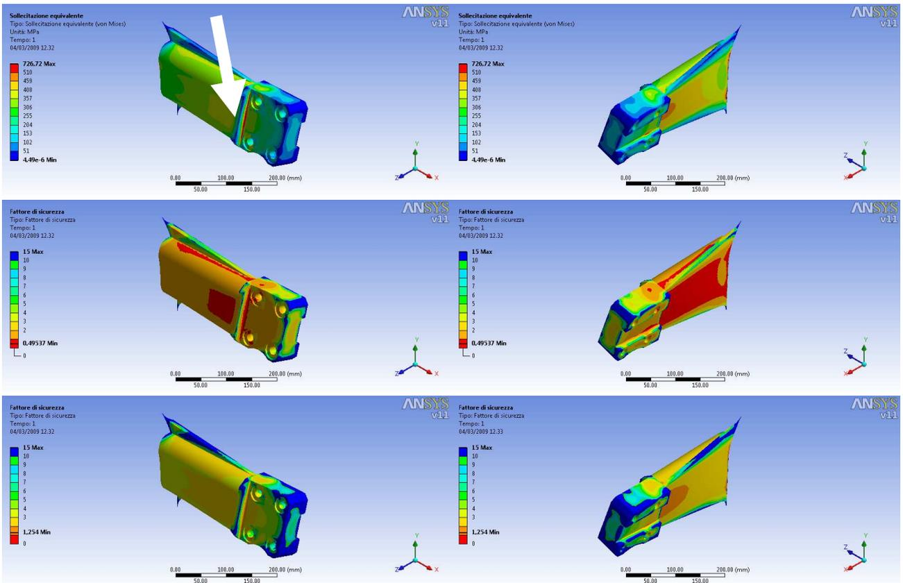
Figure 3. *Original* support arm: stress field for *exceptional* inertial load (top), safety factor for *normal* inertial load (mid) and safety factor for braking load (bottom).
