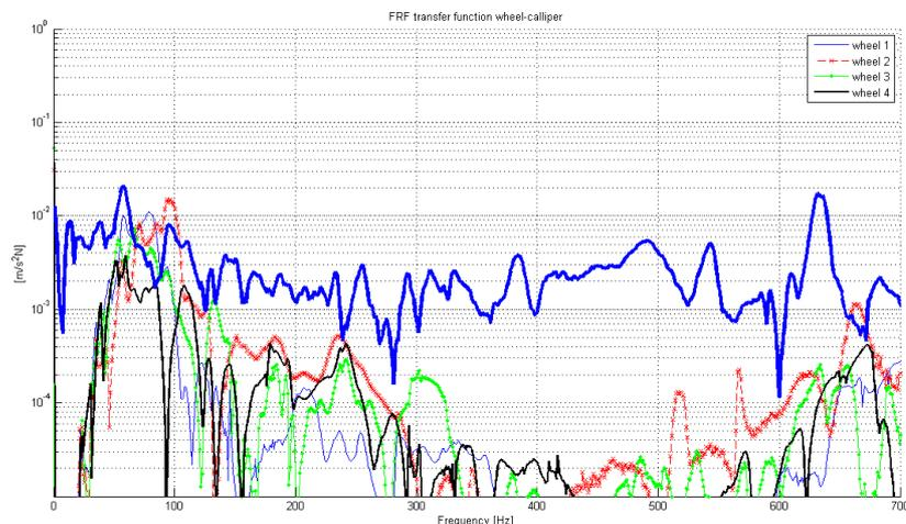
Figure 10. FRF calliper/wheel for four different wheel solutions with the redesigned brake calliper support. Blue line: without rubber element on the wheel axis, other lines: with rubber elements of different stiffness.
