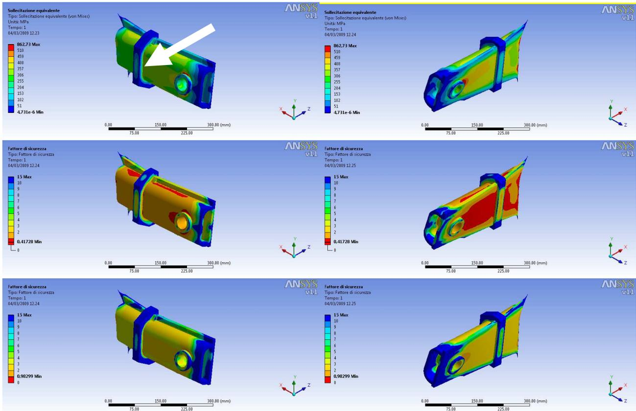
Figure 5. *Modified* support arm: stress field for *exceptional* inertial load (top), safety factor for *normal* inertial load (mid) and safety factor for braking load (bottom).
