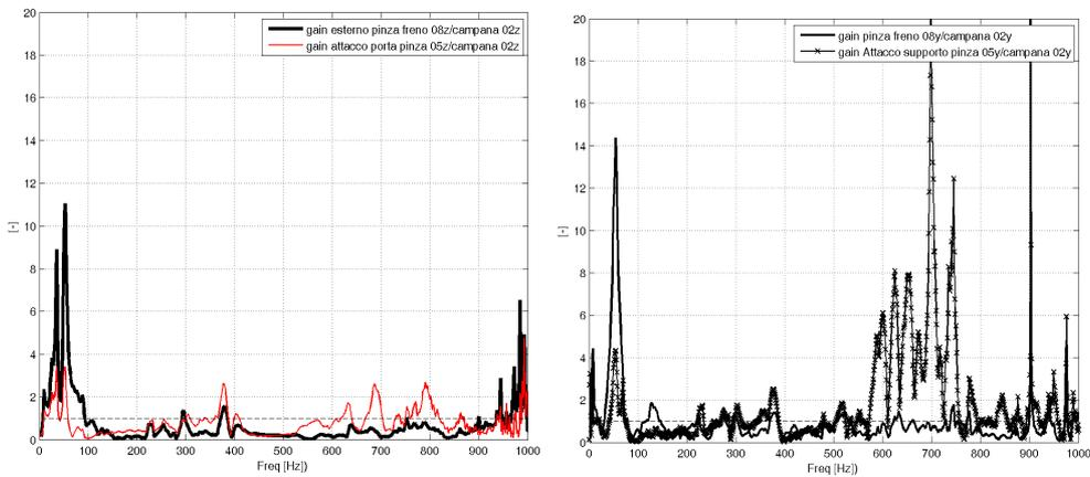
Figure 9. Gain from point 02z (bogie frame) to point 05z (calliper fixture, red line) and to point 08z (calliper side surface, black line) for vertical excitation (left). Gain from point 02y (bogie frame) to point 05y (calliper fixture, thick line) and point 08y (calliper side surface, x-x-x) for lateral excitation (right).
