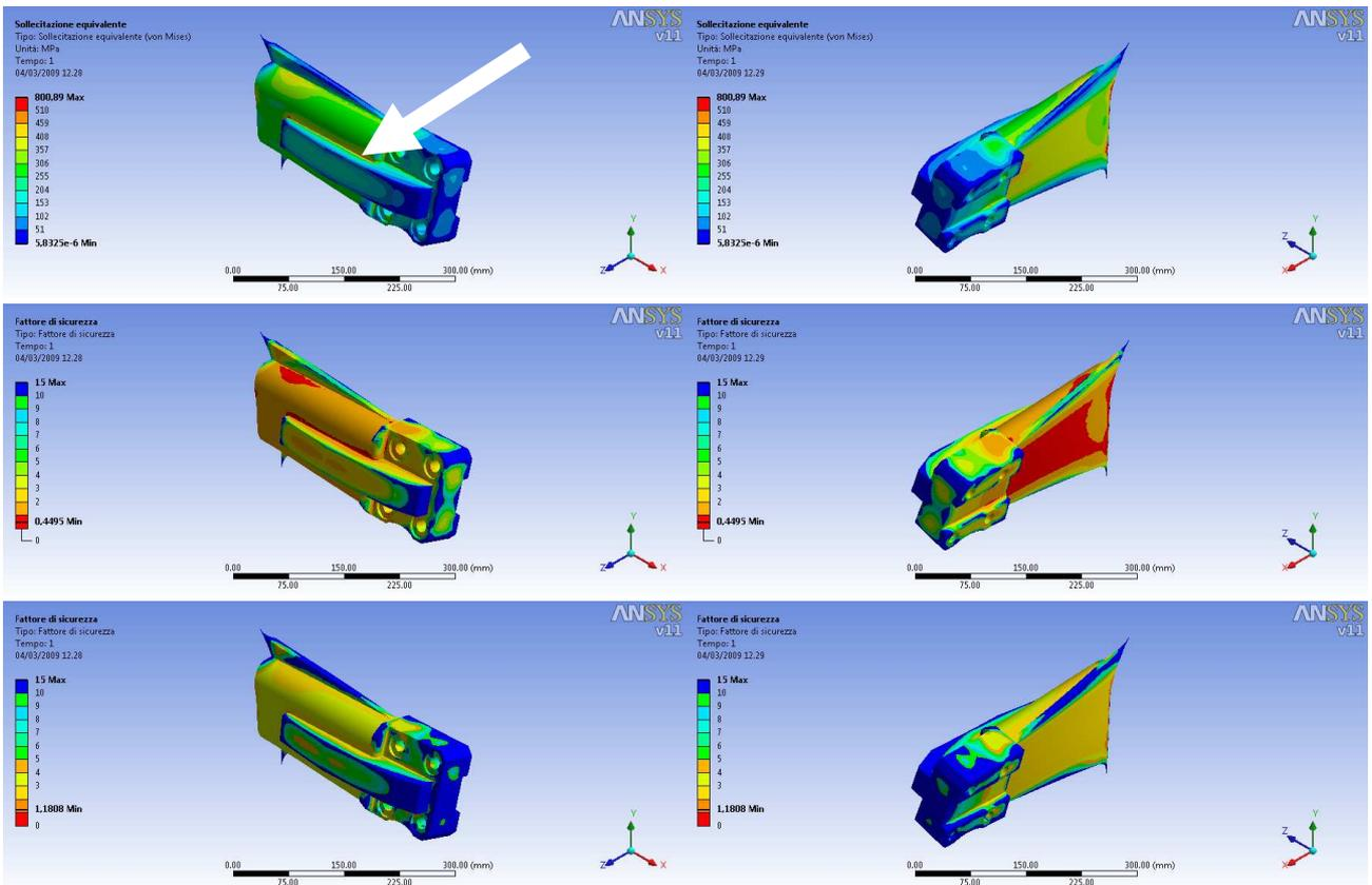
Figure 4. *Reinforced* support arm: stress field for *exceptional* inertial load (top), safety factor for *normal* inertial load (mid) and safety factor for braking load (bottom).
