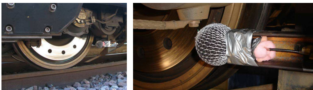
Figure 11. Powered bogie. Position of the microphone.
