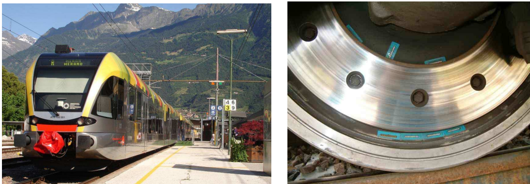
Figure 8. Position of the thermal tapes on the Syope Braw wheel to verify the maximum temperature reached in service
