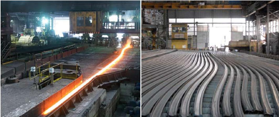
Figure 1: Rail rolling plant (left) and cooling bed (right).
