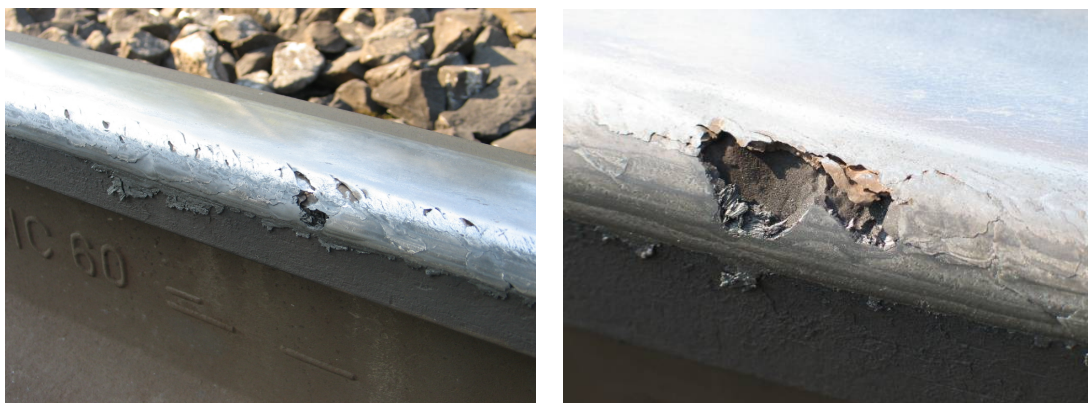
Figure 6: Extensive railhead damage shown by a heat-treated premium rail installed on the high rail in a track near Seebach Zurich. These rails were replaced with VAR110 naturally hard rails.
