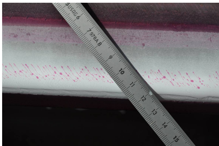
Figure 8: Head checks found on the VAR110 rail during the last test (27.04.2012). High rail, running direction left to right.
