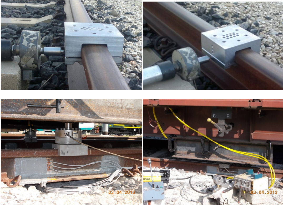
Figure 8: Devices for lateral and vertical test loads application and interface with the rail.
