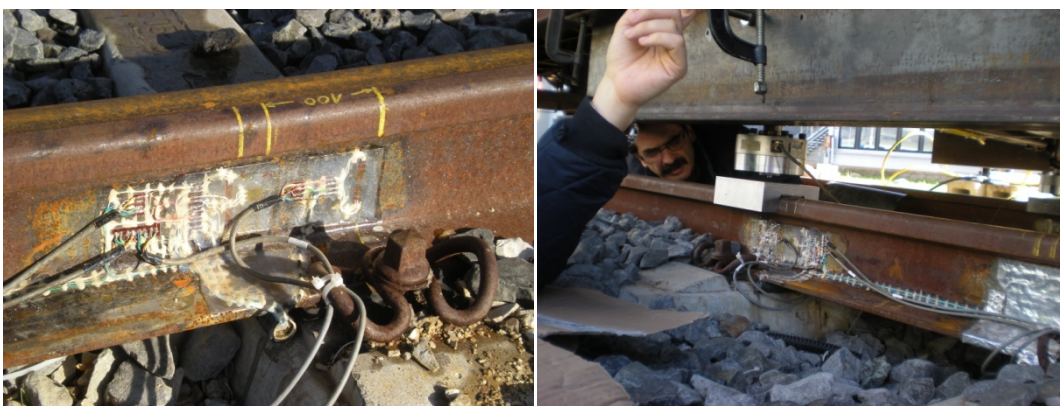
Figure 9: Left: application of ER strain gauges for Q and Y estimation. All the three methods for Y estimation are visible. Right: calibration under Q force.
