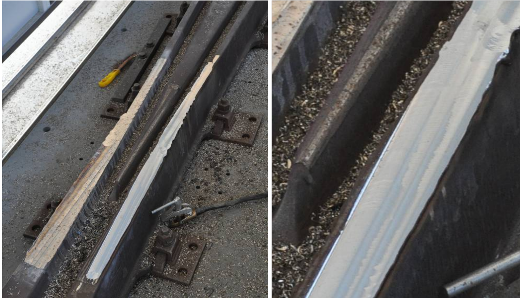
Figure 10: Example of the quality of crossing surface after final milling.
