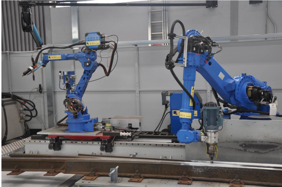
Figure 3: Welding robot R2 (Yaskawa MOTOMAN HP20D) equipped with the wire feed unit and the 19-needles scaler Beta 1944 (left). Milling robot R1 (Yaskawa MOTOMAN ES165D) equipped with measuring probe and milling spindle (right).
