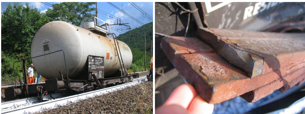
Figure 1: Railway tank derailed (left) after failure in the front left leaf spring (detailed right). Fatigue and sudden broken surfaces are clearly distinguishable.
