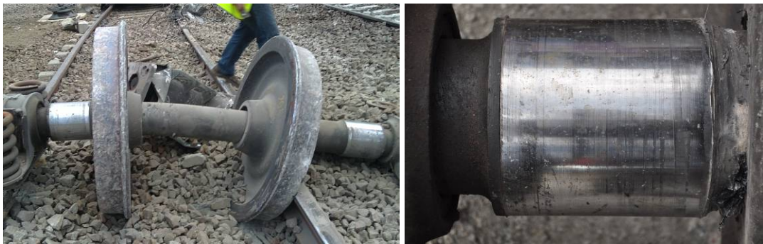
Figure 3: Displaced wheels from the wheelset on the first wheelset of the wagon (left). Aspect of the surface after wheel displacement revealed no defects or damages typical of wheels pressing off (right).
