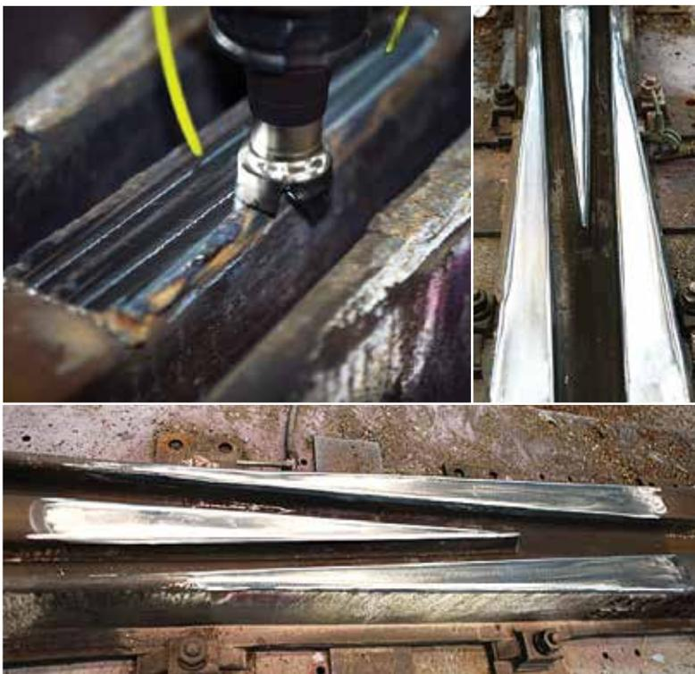
through welding, and machining to finishing, we decided to investigate the possibility of using a robotic plant for both the welding and machining phases.'
