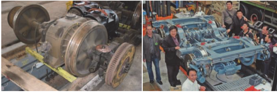
Figure 6. Two examples of brake discs mounted on the axle ends. The bogie to the right has internal bearings.
