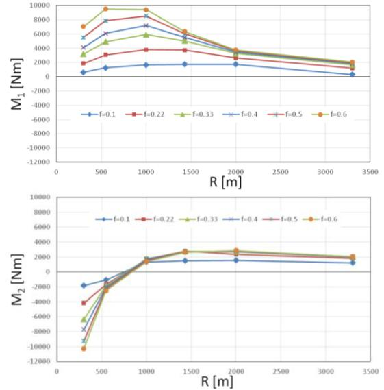
Fig. 5. Torque acting on the leading wheelset M1 (top) and trailing wheelset M2 (bottom) for different  $f$  values for the standard ERRI wagon.
