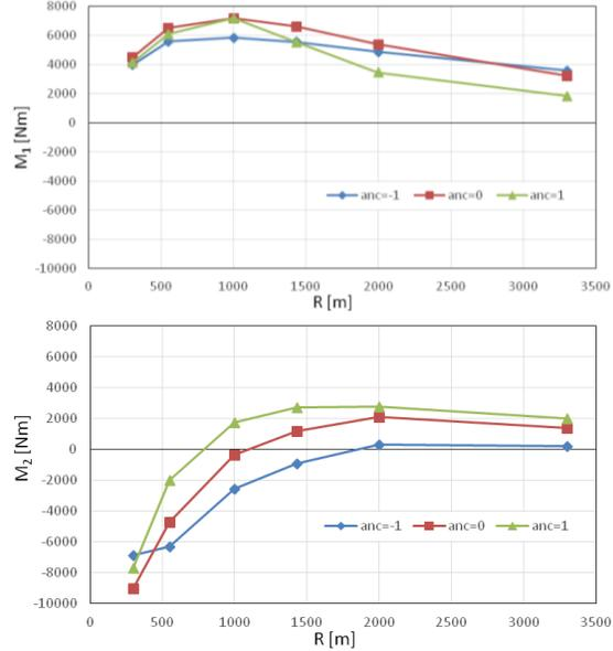
Fig. 3. Torque acting on the first two wheelsets of the ERRI Wagon for  $f=0.4$  as a function of  $a_{nc}$ .
