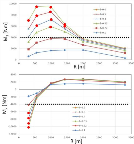
Fig. 7. Zoom on the torque on both wheelsets (see Fig. 5). Torque limit (dotted line) was set to 4000 Nm. Red dots indicate where torque reduction is larger than 33%.
