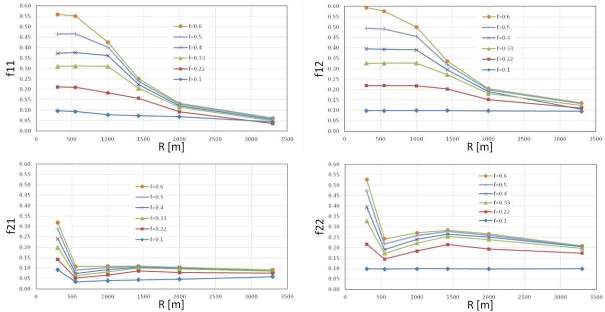
Fig. 6. Utilized adhesion for the four wheels of the leading bogie of standard ERRI wagon.
