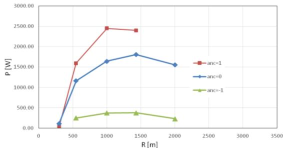
Fig. 10. Power dissipated in the front wheelset (torque limiter set to  $M_{lim}=4000$  Nm) for different  $a_{nc}$  conditions and  $f=0.4$ .
