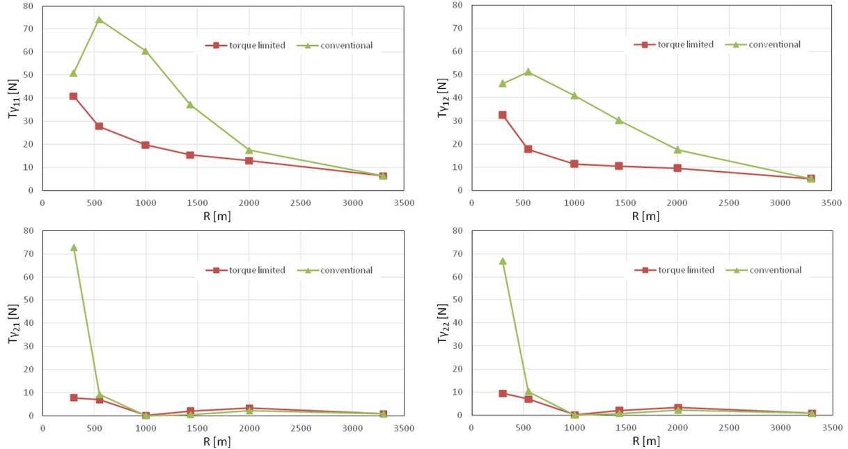
Fig. 8. Longitudinal wear number  $T_{x\gamma}$  for all the wheels of the ERRI wagon in the original configuration and with the torque limited to 4000 Nm.
