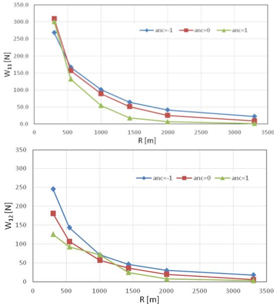
Fig. 2. Wear numbers  $W=T\gamma=T_x\gamma_x+T_y\gamma_y$  for the outer wheel ( $I1$ , top) and the inner wheel ( $I2$ , bottom) of the first wheelset of the ERRI Wagon for  $f=0.4$  as a function of  $a_{nc}$ .
