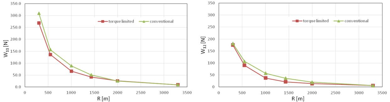
Fig. 9. Total wear number  $T_{x\gamma}+T_{y\gamma}$  for the front wheels 11 and 12 of the ERRI wagon in the original configuration and with the torque limited to 4000 Nm.
