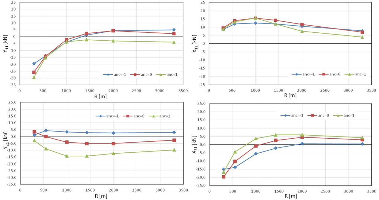
Fig. 4. Lateral forces (left) and longitudinal forces (right) for the leading (top) and trailing (bottom) wheels of the first bogie of the ERRI wagon.
