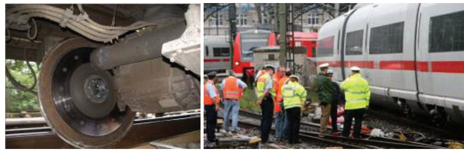
Figure 22: Broken axle of the IC518 ICE3 train in the Köln main station, 9.7.2008. Left: the broken driving axle seen from the internal side. Right: investigators looking at the derailed train [24]
