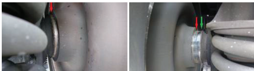
Figure 30: Both wheels displaced of a freight wagon in Verona (13.02.2015)
