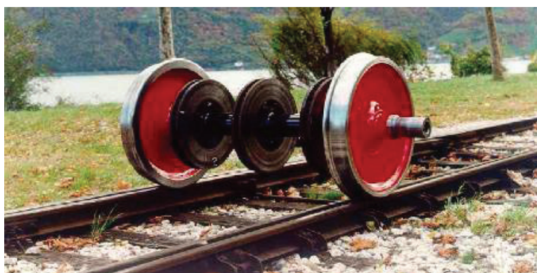
Figure 11: Application of damping treatment on the wheel web of a high-speed train wheelset in order to reduce wheel vibrations and therefore emitted noise ( Syope treatment, Lucchini RS, [4])
