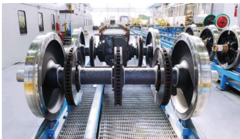
Figure 12: Application of anti-ballast shock protection layer on the axle ( Lursak treatment, Lucchini RS [4], [11])
