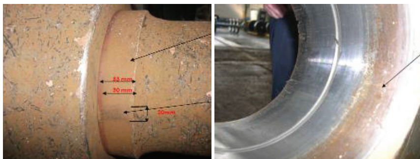
Figure 29: Displaced wheels towards the axlebox of a passenger car (left). Aspect of the wheel bore after dismounting during the investigations (right) [40]
