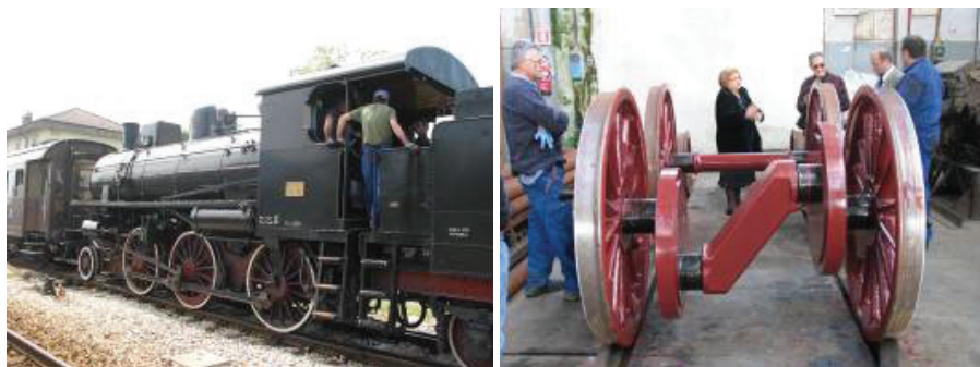
Figure 3: Class 625 locomotive of the FS (Italian State Railways) pictured during a revival train (Bornato, Italy, 15.05.2005). Driving and coupled wheelsets pictured at the Historical Rolling Stock depot in Pistoia, Italy. Journal seats and crankpins for driving rods are clearly visible. Both photos by the Author
