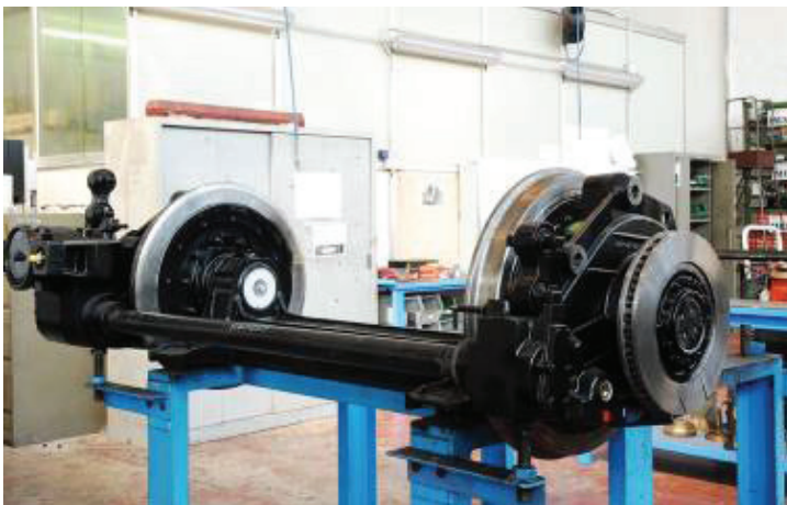
Figure 18: Driving axle of the AnsaldoBreda Sirio vehicle. The shaft connecting the two wheels is in the foreground [4]
