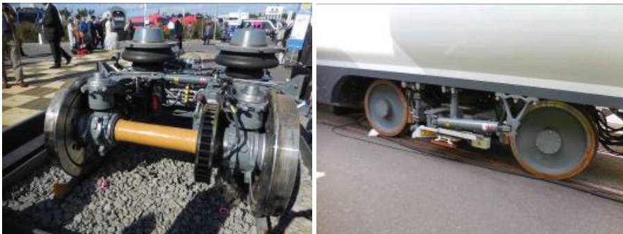
Figure 14: Detail of the trailing bogie Bombardier FlexxECO for ICx (left) and Siemens Desiro City Thameslink (right) (Innotrans 2014, Berlin)
