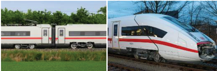
Figure 13: The new ICx trainset for German Railways DB. Left: a trailing bogie ( FlexxECO made by Bombardier Transportation) and a motor bogie (made by Siemens AG) on two adjacent cars. Right: the driving trailer car equipped with FlexxECO bogie
