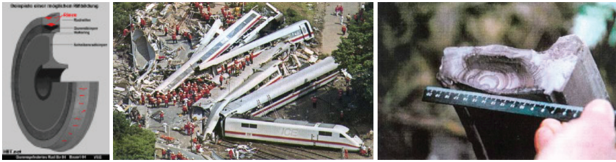
Figure 27: Sketch of the BA 064 wheel (left, from http://www.ndt.net/news/2000/eschedec.htm ). An image on the aftermath of the disaster (centre, from http://uncyclopedia.wikia.com/wiki/File:Eschede-1.jpg ). Fractured tyre section (right, from http://www.soue.org.uk/souenews/issue6/jenkinlect.html )
