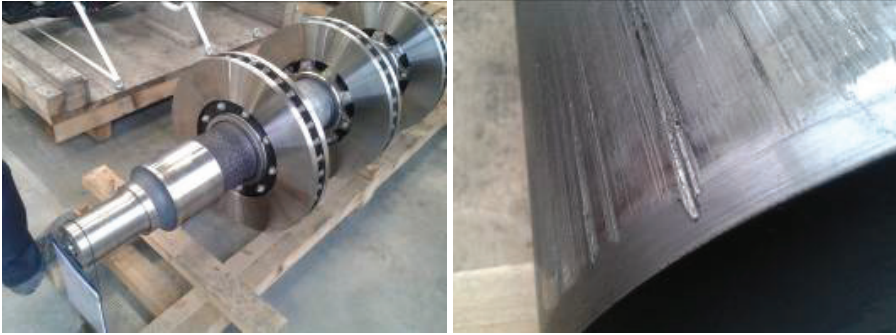
Figure 31: Consequences of a misfit of a wheel on a wheelseat. The deepest grooves are originated by the wheel removal process (photo by the author, 2013)
