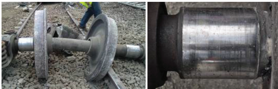
Figure 28: Displaced wheels from the wheelset on the first wheelset of the wagon (left). Aspect of the surface after wheel displacement revealed no defects or damages typical of wheels pressing off (right) [39]
