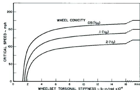
Fig. 4 The effect of wheel conicity on critical speed with variable wheelset torsional stiffness. Conversion factors: (n-m/rad) = (.113) (lb-in./rad); (kph) = (1.61) (mph)
