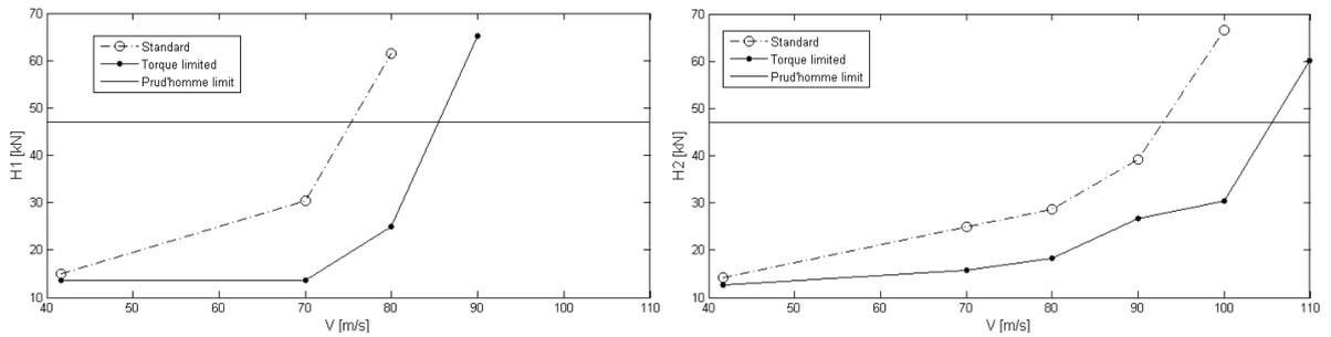
Figure 13. Track shifting forces of a standard wheelset and the torque limited wheelset. Both first (left) and second (right) axles are shown.
