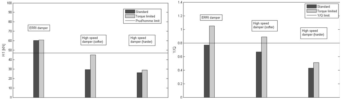
Figure 15. Comparison of  $\Sigma Y$  of the first wheelset (left) and  $Y/Q$  of the first external wheel (right) for a standard wheelset and a wheelset equipped with torque limiter and an average flexible axle ( $D = 140 \text{ mm}$ ,  $d = 80 \text{ mm}$ ,  $l = 2000 \text{ mm}$ ).
