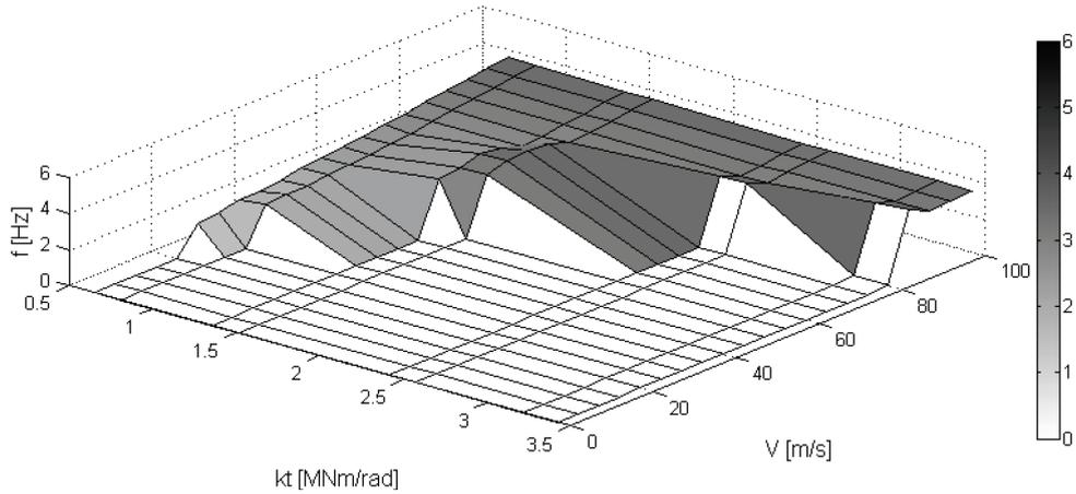
Figure 12. Frequencies of the lateral oscillation of the first wheelset equipped with the torque limiter.
