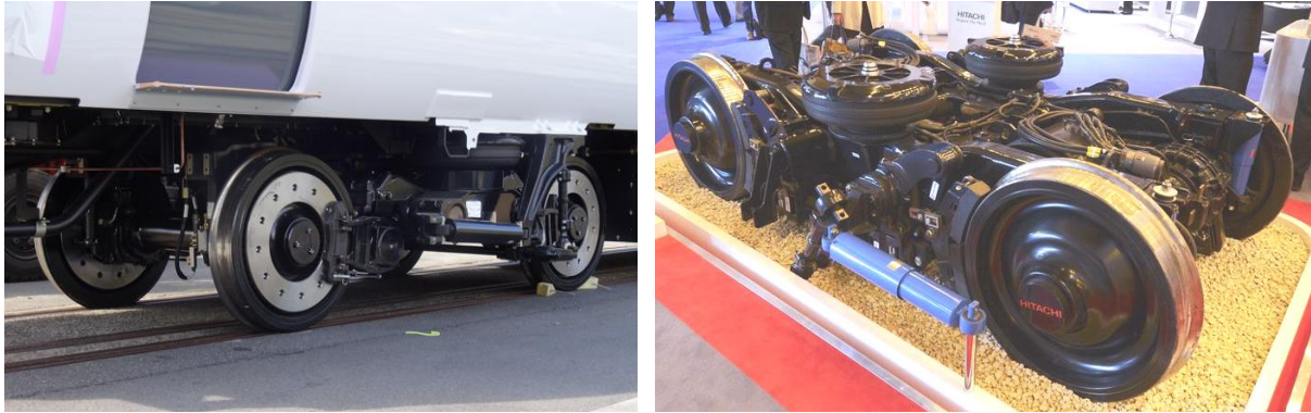
Figure 5. Hitachi inside frame trailer bogie for IEP trains (left). An inside frame motor bogie on display at the trade fair Railtex 2013.
