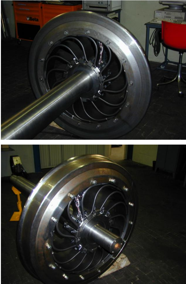
Figure 1. The “springy wheel” developed by Sulzer in the ‘90s pictured in the Lucchini Sidermeccanica plant.
