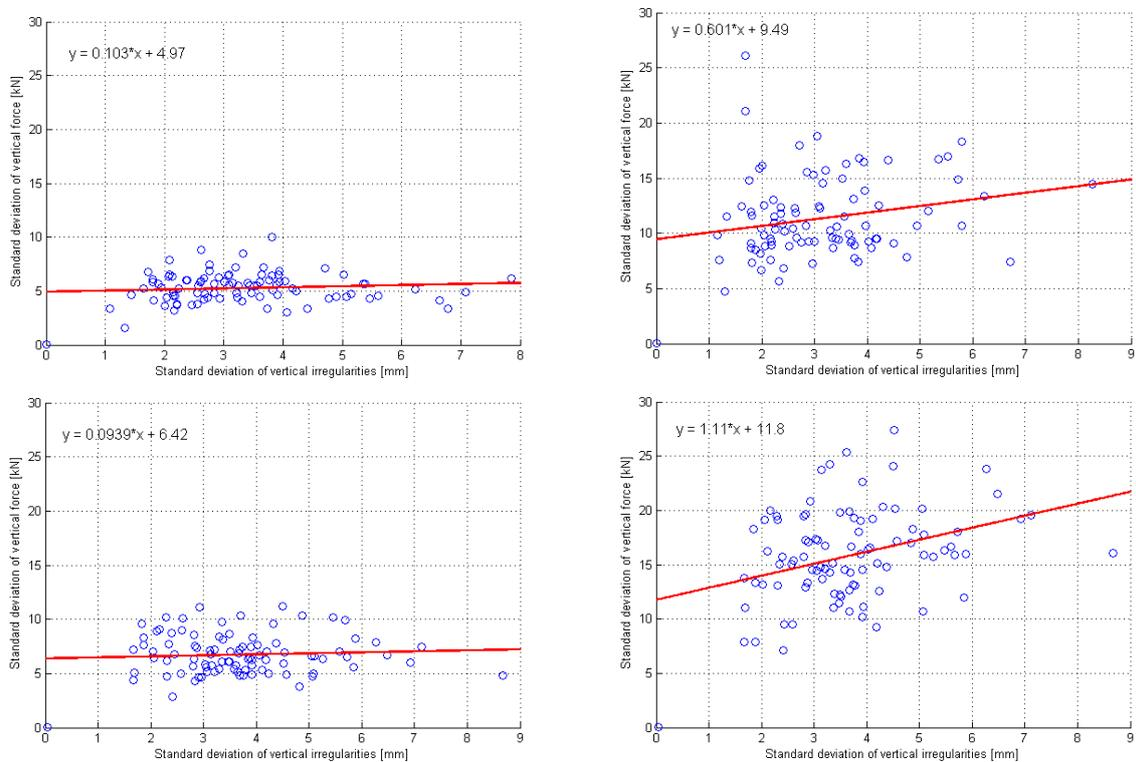
**Figure 10** Standard deviation of the vertical dynamic force over 100 m long track sections for the empty wagon (left) and for the laden wagon (right) plotted against the standard deviation of vertical irregularities at the speed of 120 km/h (above) and of 145 km/h (below). Red lines are the best fit linear regressions.
