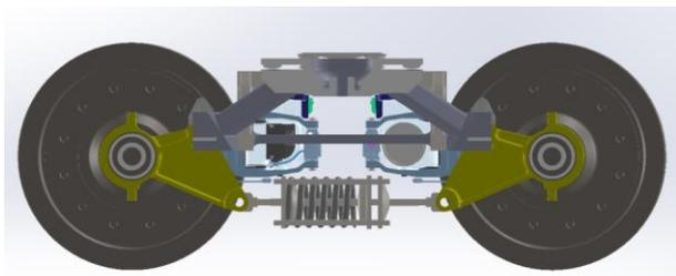
Figure 2 Primary suspension arrangement of the modified bogie from an inside view. One progressive coil spring is used on each side.
