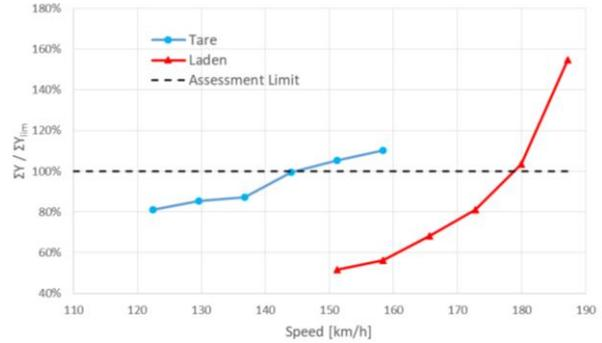
**Figure 6** Stability assessment in tare condition and laden condition.
