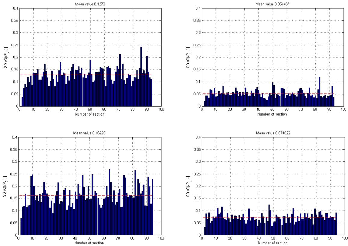
**Figure 9** Standard deviation of the vertical dynamic force over 100 m long track sections for the empty wagon (left) and for the laden wagon (right) at the speed of 120 km/h (above) and of 145 km/h (below). Dashed red line represent mean values.
