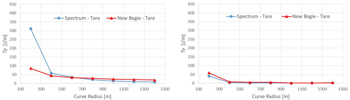
Figure 12 Front wheelset (left) and rear wheelset (right)  $T_\gamma$  comparison of leading bogie of the spectrum vehicle (from [9]) with the new bogie (tare condition, zero cant deficiency).
