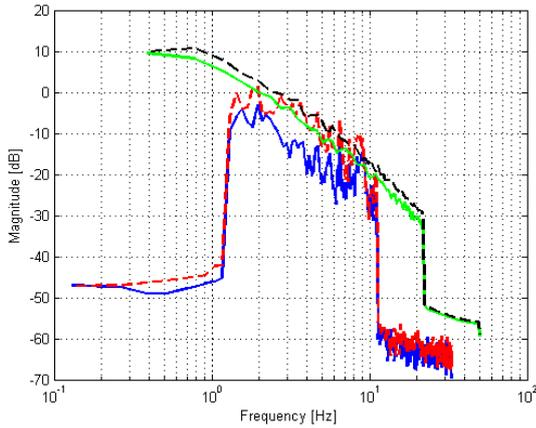
**Figure 4** PSD distribution of lateral (alignment, solid blue) and vertical (longitudinal level, dashed red) for measured defects and the corresponding ERRI “High Level” irregularities lateral (solid green) and vertical (dashed black).
