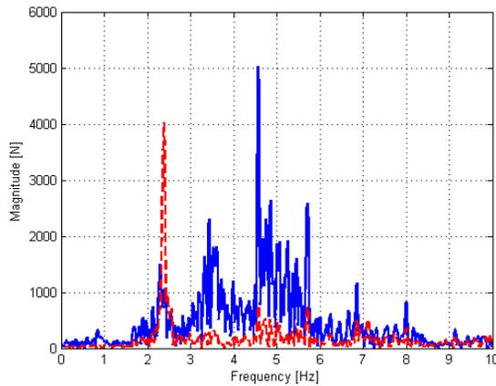
Figure 7 Vertical frequency response for empty (dashed red) and laden (solid blue) conditions
