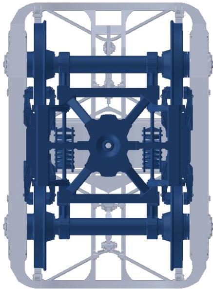
Figure 1 Schematic representation of the overall dimensions of an Y25Ls(s) bogie (grey), compared with the innovative inside frame bogie (blue).
