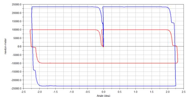
Figure 3 Yaw resistance vs. the yaw angle of the bogie for an empty wagon (red) and for a laden wagon (blue).
