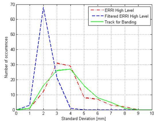
Figure 8 Number of occurrences of the standard deviation of vertical ERRI High Level defects as generated (red), filtered in the *D1* wavelength (blue) and the *Track for Banding* distribution (green).
