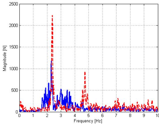
**Figure 5** Lateral frequency response for empty (dashed red) and laden (solid blue) conditions
