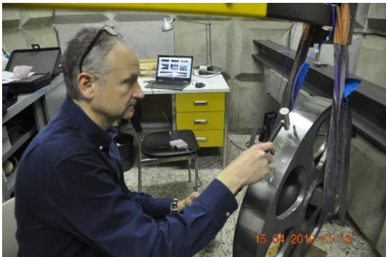
Fig. 12 FRF measurement to validate the FEM model and to estimate damping properties of ADI cast iron.
