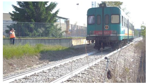
Fig. 13 Pass-by noise measurements at 80 km/h near Rovato (Italy) on 16 May 2019.
