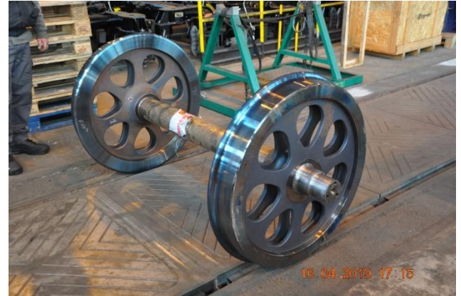
Fig. 8 First wheelset assembled with ADI cast iron wheel centres.
