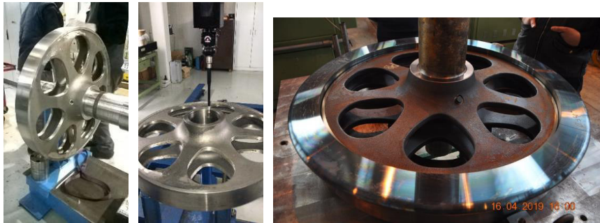
Fig. 13 Left: first mounting on an axle. Mid: CMM dimensional check. Right: first Liberty Wheel assembly with the tyre.
