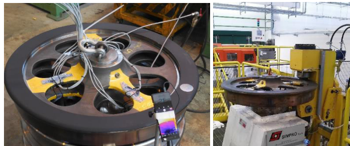
Fig. 15 Measuring the strains in the spokes by means of ER strain gauges during cooling of the tyre (left). The Liberty Wheel under test mounted in the full-scale facility (right).
