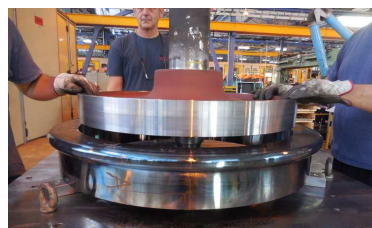
Tyred wheels: Tyre fitting on a wheel without abutment and Gibson ring (Comafer, October 2018).
