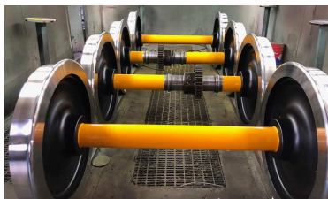
Tyred wheels: Set of finished tyred wheelsets (two driving, two trailed) for ALn 668.
