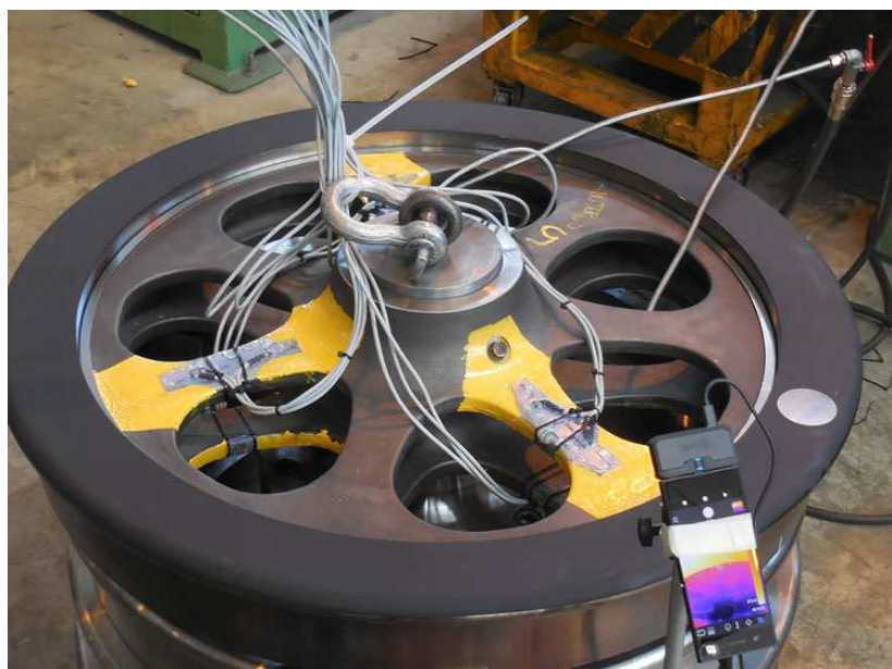
Liberty Wheels: Checking stresses and strains during tyre cooling of the first Liberty Wheel.
