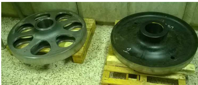
Liberty Wheels: Comparison of original and Liberty Wheel centre (-50 kg).
