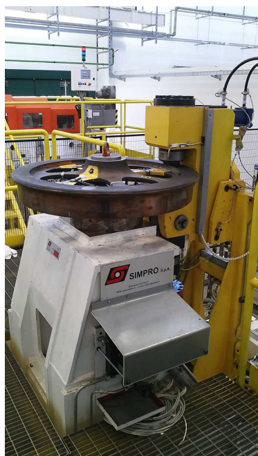
Liberty Wheels: Full-scale fatigue tests (Italcert Labs, May 2019).
