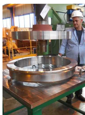
Tyred wheels: Shrink-fitting a fully machined tyre on a dovetail wheel centre. Note the absence of any abutment and Gibson ring.
