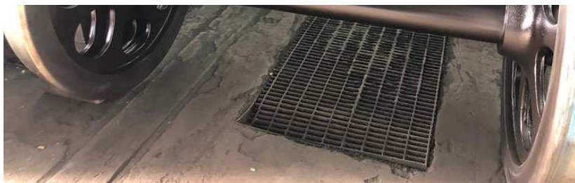
Liberty Wheels: Set of finished tyred wheelsets (two Liberty Wheels in front) for ALn 668 (April 2019).
