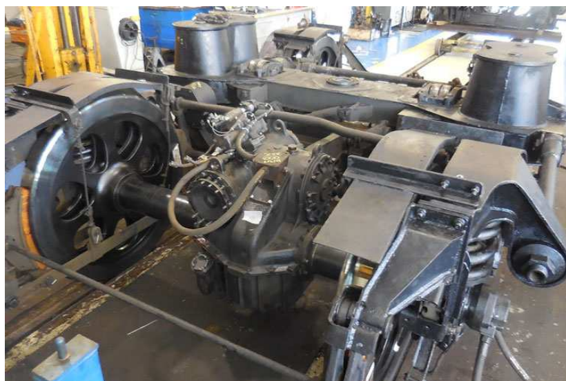
Liberty Wheels: ALn 668 DMU bogie equipped with Liberty Wheels (May 2019).
