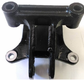
Fig. 21 Left: a modified support with an 80-mm welded stiffener. Right: measurement of the point FRF on both original and modified support
