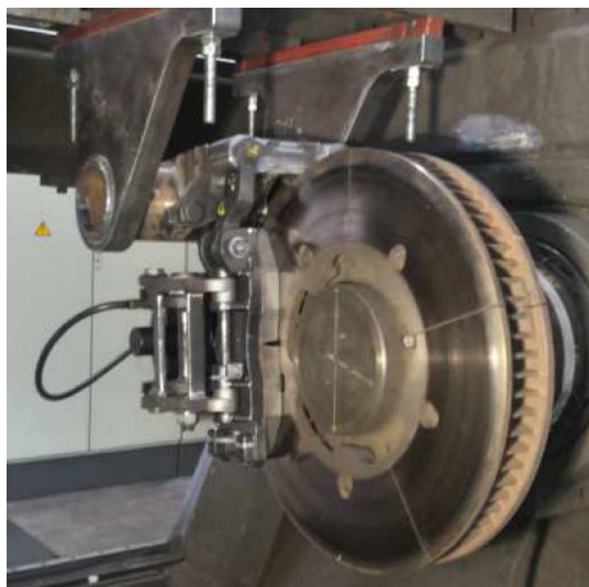
Fig. 2 Brake unit installed on the brake test bench
