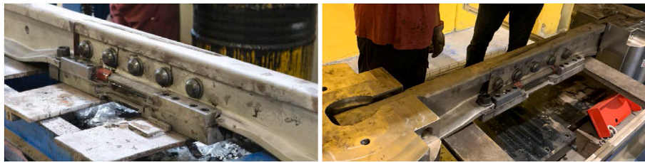
Fig. 18. First ABJ prototype just after the assembly (left) and placed into the pull-apart machine (right).
