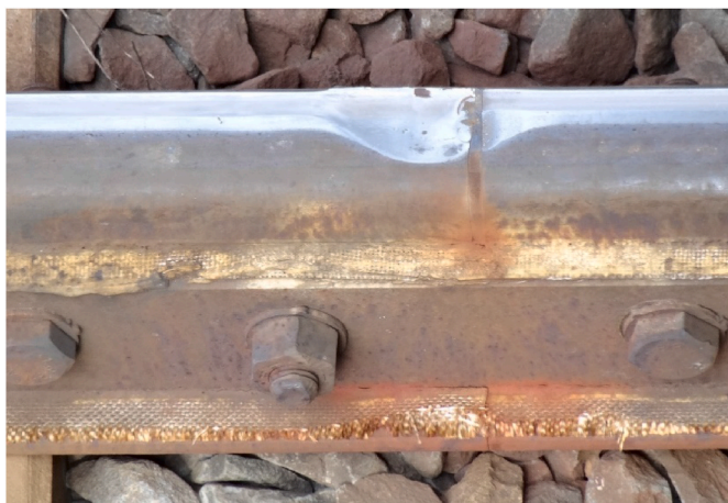
Fig. 1. IRJ with heavy plastic deformation generated by dynamic forces at each wheel passage. Insulating elements are clearly damaged (Photo by the authors).
